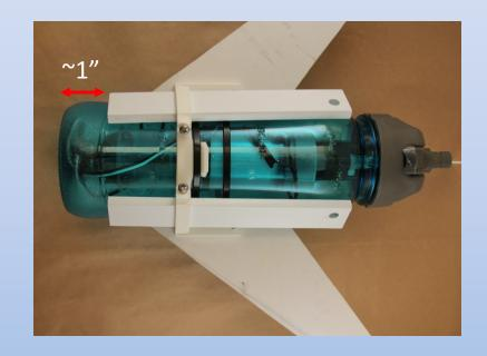
The two 6" bars fit in slots of the wing yoke on the underside of the glider. (The opposite side of the NATHAN label.) Slide one bar into each slot about 1" from the nose of the glider. Secure the bars in place with #6 screws from the Buoyancy Engine bag.
