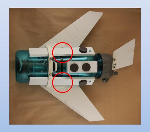
Sometimes the pitch is fine and ballast is needed just to sink the glider when the buoyancy engine draws in water. More magnets can then be added symmetrically to a pitch neutral location, usually under the wings.
