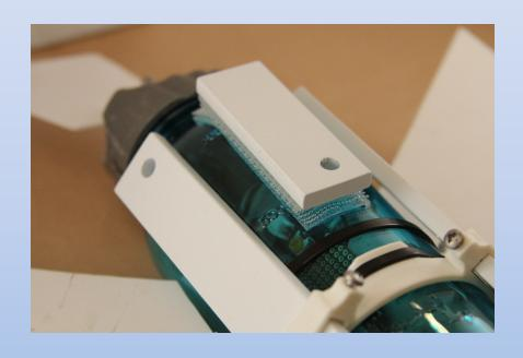
Matchup the Dural-Lock strips and press the small bar into position between the two larger bars.
