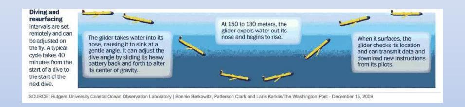
The graphic above shows an ideal cycle or yo for a commercial ocean-going glider. Good forward progress is achieved on both dive and rise cycles. SeaGlide works the same way; it must sink & pitch down on the dives and float & pitch up on the rises.
