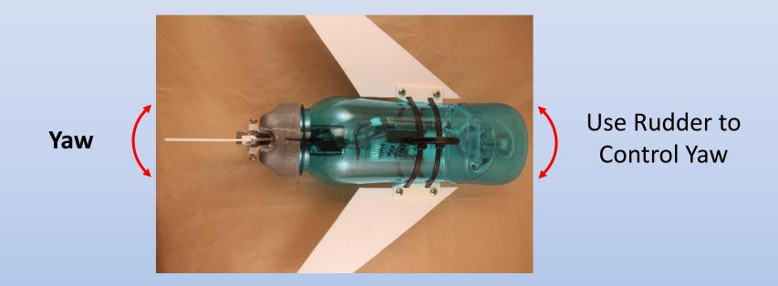
The manual rudder on SeaGlide can be used to help direct the glider straight or to turn left or right. It enables the glider to fly in circles or around objects such as a buoy marker.
