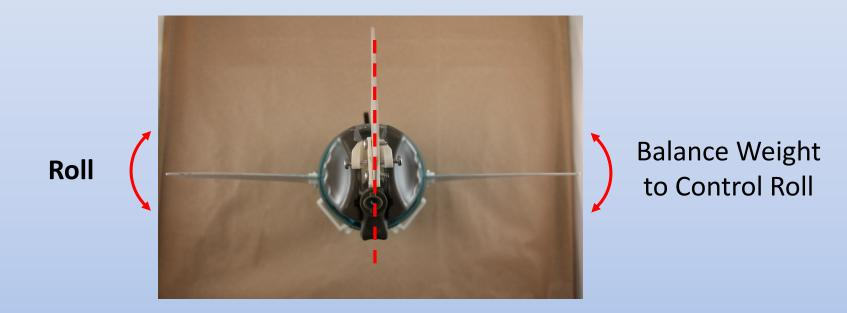
A weight difference between the two halves of the glider can cause roll and a wing to dip, leading to an unwanted turn. Make sure the buoyancy engine is centered in the bottle. If the servo end is off to one side at the nose of the glider, thump the opposite side with the heal of your hand to center it.
