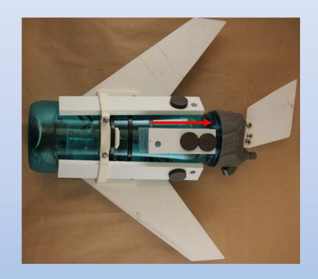
Often a glider flies well when diving, but does not pitch up in the rise cycle. It may float straight up with no forward progress, or even go backwards. To correct this, move magnets and/or small bar backwards towards the tail. If ballasting is way off, you may need to move the two large bars back. This may be required if you attach an action camera to the front of the glider.
