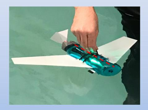
With the buoyancy engine plunger centered and the syringe full of water, the glider should barely float and be level or a little nose up in the water. Only a ~½"-wide strip at the top of the bottle should protrude above the waterline.
