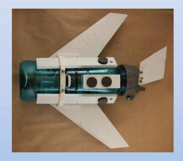
Stick small magnets on the steel bars for additional ballast.
