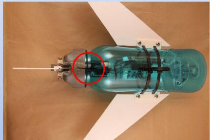
With the cap installed securely, mark the position on both the bottle and cap with a marker. If you match these witness-marks each time you close the bottle, you can ensure that your rudder is perpendicular to your wings every time. This will help your glider fly straight.
