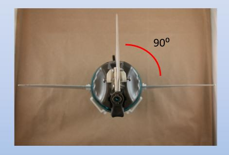
To avoid unwanted turning due to malalignment of the wings and rudder, rotate the wing yoke and wings so that they are at a 90° angle to the rudder.
