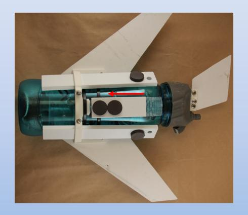
If the glider is not pitching down and diving well, you can move magnets and/or the small bar forward towards the nose of the glider. Usually it's not necessary to move the large ballast bars.
