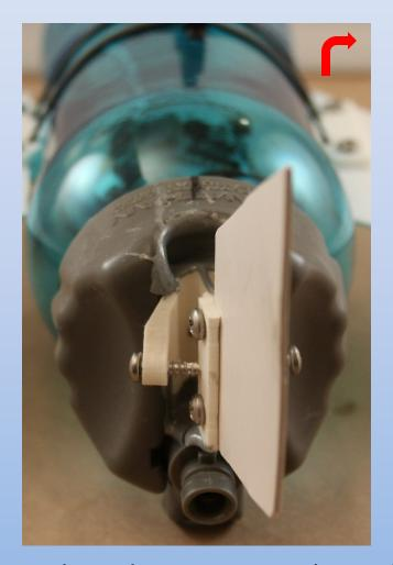
Adjust set screws, loosen one and tighten the other, to move the rudder.
