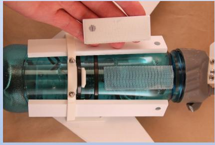
Cut a Dura-Lock strip to the length of the small bar. Remove the backing and stick it to the bar. Cut another Dura-Lock length to fit in space between the two long bars and the wing yoke and cap. Remove the backing and secure midway between the bars as shown.
